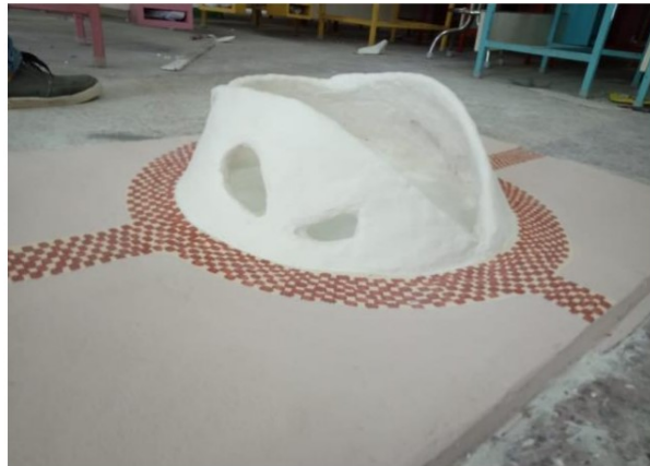
Ferro cement model lay to set @E210 - School of Architecture
