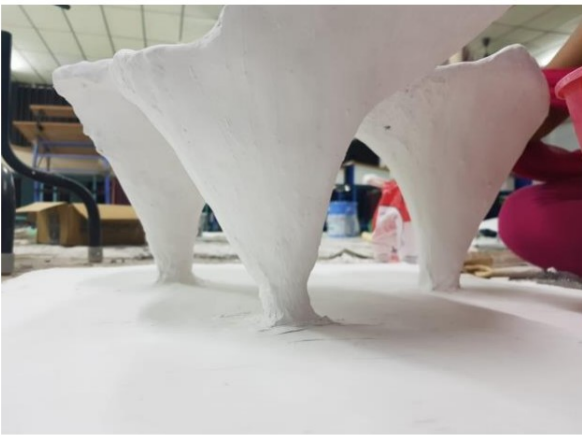
Ferro cement model lay to set @E210 - School of Architecture
