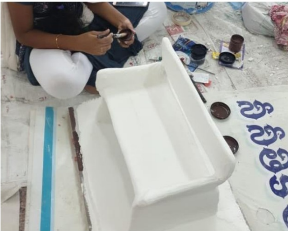
3rd year students working on the plastering of the ferro cement model on 15-09-2019 @E210 - School of Architecture
